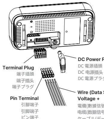
Choose only one of the two power supply options, either the DC adapter or the DC source via terminal plug, but NOT both at the same time.
