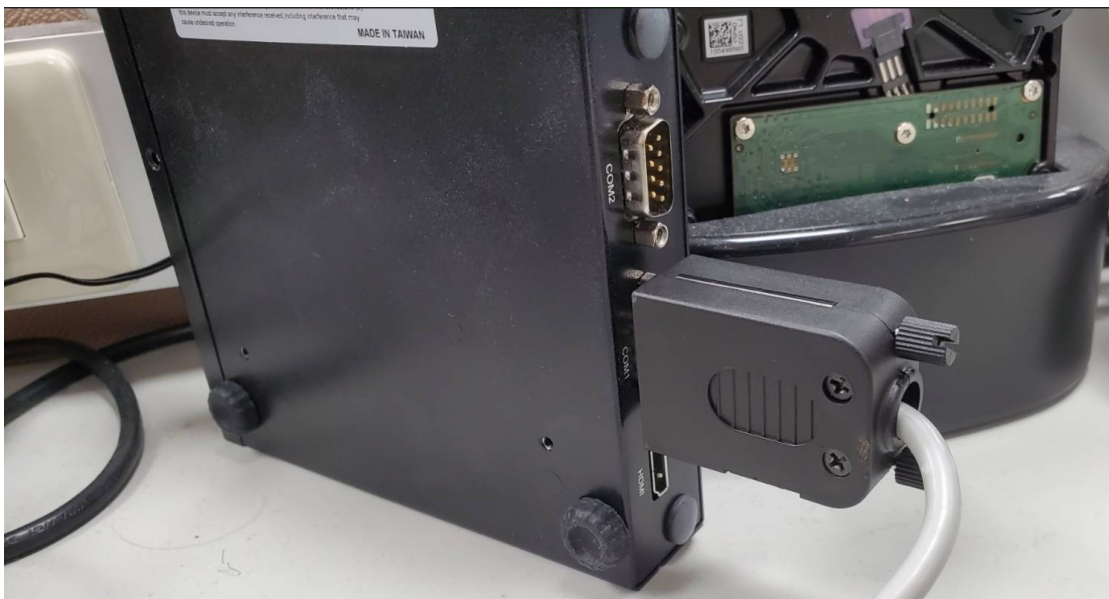
6. Install connector on the COM1 of UNOCentral
